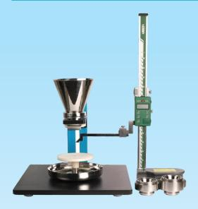
The Angle of Repose is the angle (relative to the horizontal base) of the conical pile produced when a granular material is poured onto a horizontal surface. It is related to the density, surface area and coefficient of friction of the material concerned.
